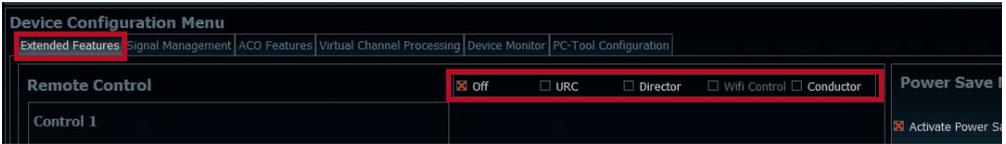
If the VCP is **not activated**, the subwoofer remote control of the PP 86DSP MK2 is permanently assigned to the output channels G and H. In this case it does not matter which output is named “Subwoofer” in the IO routing matrix.
