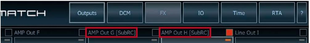
When VCP is **activated**, the subwoofer remote control is tied to the output channels that are supplied with one of the two virtual subwoofer signals (“Subwoofer 1” or “Subwoofer 2”) in the “Virtual to Output Routing” matrix. This can be any combination of output channels.
