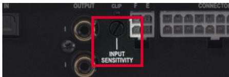
This is not a volume control; it's only for adjusting the amplifier gain. The setting of the control only affects the highlevel inputs.
